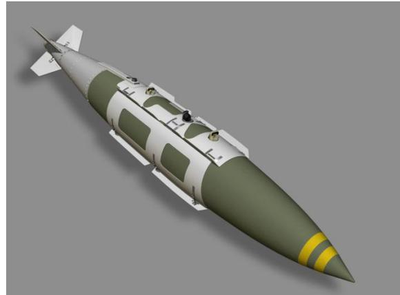
Because of its modular design, the JDAM family of weapons includes affordable add-on options to increase the warfighter’s flexibility and reach. A Laser JDAM sensor allows JDAM precise prosecution of moving, relocatable and maritime targets. JDAM Extended Range (JDAM ER) incorporates a low-cost wing set to extend JDAM’s standoff range from approximately 15 miles to more than 45 miles.
